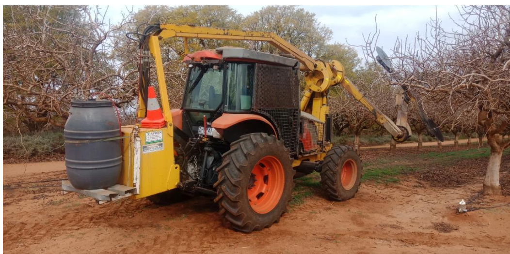
The 4-bladed hedging/tipping/topping/skirting machine.
