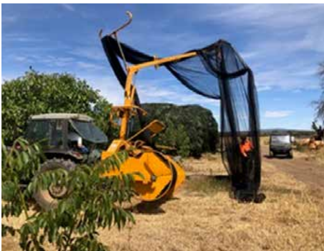
Photo supplied by Mark Jankelson – Boonderoo - Redesdale Victoria. Purpose built netting equipment for installing and removal of bird netting.
