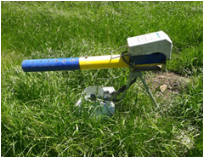
Wellwood 2020. One of 3 Zon brand Gas cannons with extendable tube to vary the amount of gas build-up inside the tube for a louder "Bang". Effective range 200m . Currently not in use with the long grass surrounds
