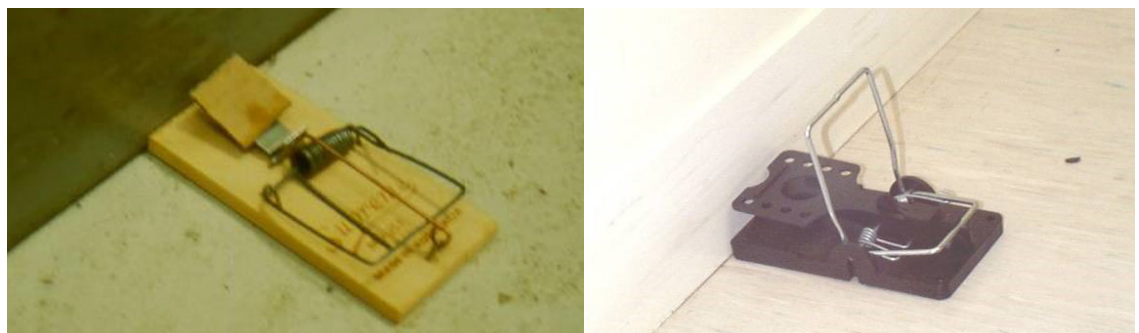
Figure 3: Kill traps. (a) Mouse Trap: “Supreme” - 10cm long, set against of all. Surface of trigger has been enlarged using leather soaked in linseed oil. (b) Strong plastic moulded rat trap - 14cm long. **NB** Photos not to scale
